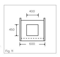
400mm wide and a minimum of 15mm high to allow air to pass under the unit. Alternatively cut a section 400 x 450 mm in the base of the carcass as indicated in fig. 11. Failure to allow adequate ventilation to the appliance may result in overheating or damage to adjacent units and could invalidate the warranty.
