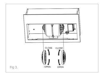
Please note thatcharcoal filters are only required when the extractor is being used in recirculation mode. Charcoal filters are not supplied and are available to purchase from our Customer Care team.
