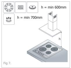
If the instructions provided with your gas hob dictate that the required distance between hob and extractor must be greater than 700mm then that is the distance that should be observed; this is a legal requirement and failure to comply with the regulations may lead to your hob being disconnected from the mains gas supply, and the installation reported to RIDDOR. Any heights measured are from the top of the gas burners.
