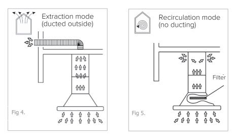
Note that when used in recirculation mode, the extractor will only remove grease and odours from cooking. It will not remove steam.
