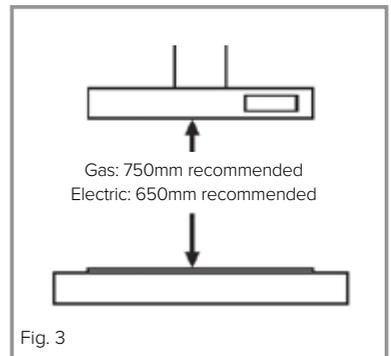
If the instructions provided with your gas hob state that the required distance between the hob and extractor must be greater than 700mm, then that is the distance that should be
