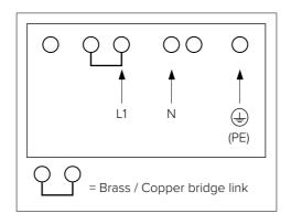
• Ensure that the brass links are securely fitted. Failure to do so may prevent the hob from operating correctly.
