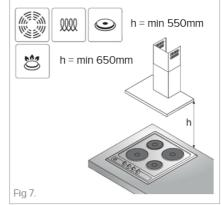
If the instructions provided with your gas hob state that the required distance between the hob and extractor must be greater than 650mm, then that is the distance that should be observed; this is a legal requirement and may lead to your hob being disconnected from the gas supply and the installation being reported under RIDDOR (The height should be measured from the top of the burners).
