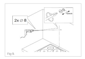
Secure the chimney fixing bracket to the wall directly below ceiling height, ensuring it is centrally located in reference to the extractor mounting holes shown in fig 8. Drill two holes and secure the chimney in place using suitable wall fixings and screws.
