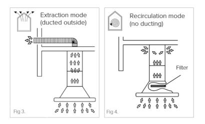
Note that when used in recirculation mode, the extractor will only remove grease and odours from cooking. It will not remove steam.
