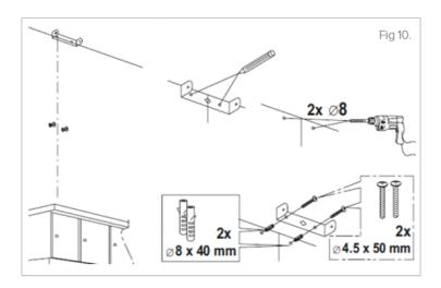
If the extractor is to be operated in extraction mode using ducting then a hole will need to be drilled in the rear wall or the ceiling to accommodate the 150mm ducting required.
