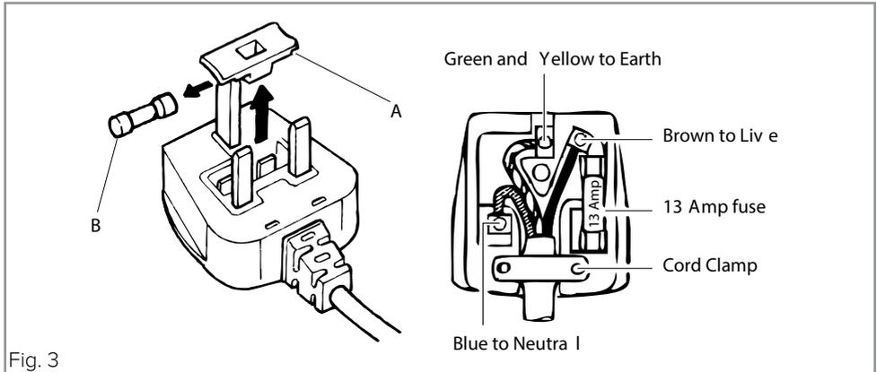
The mains lead of this appliance has been fitted with a BS 1363A 13 Amp fused plug. To change a fuse in this type of plug, follow the steps below:
