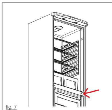
5. Unscrew the upper hinge pin and screw it into position of the left hand side (fig. 8).
