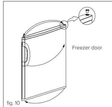
8. Rotate the central hinge 180°. Assemble the fridge and freezer doors with the central hinge and replace the doors. Secure the central hinge using the screws removed in step 1.
