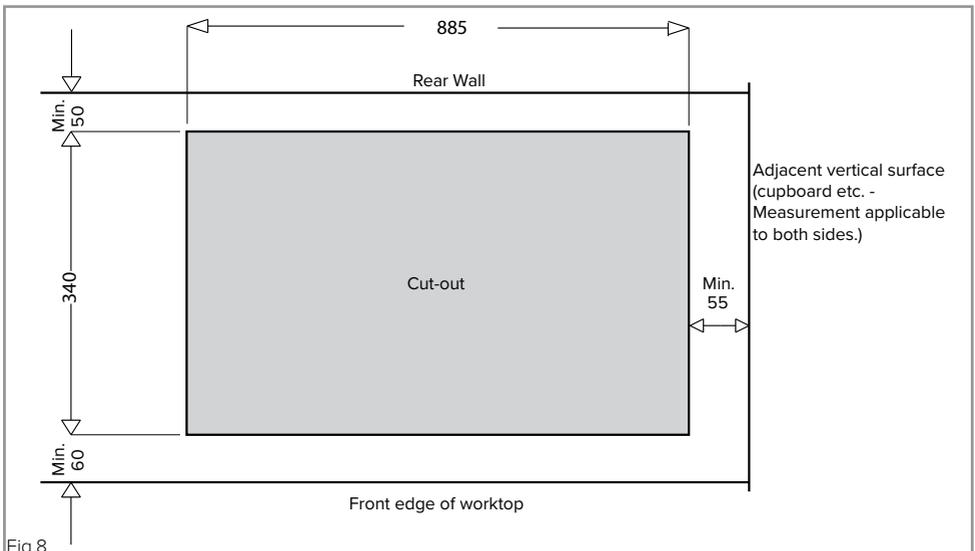
2. Make sure that the worktop is clean and dust free and insert the hob into the cut-out opening. Press the hob firmly into place so that the seal connects with the worktop (Fig. 7).
